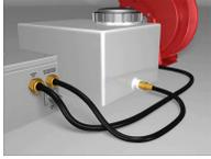
Use the appropriate 3/8” tubing to connect the Cleaning Solution Tank to the Control Box. Cover the tubing with tubing protector before attaching the ends to the DOT approved connectors. Secure with tie-downs.
