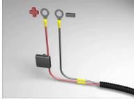
Fit the 16 gauge wire from the Control Box to the sewer truck’s battery. Connect the non fused end of the wire to the Control Box. When completed, connect the fused end to the sewer truck’s battery. Connect the red wire to the positive battery terminal and the black wire to the battery’s negative terminal.
