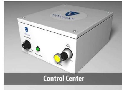
The Vanguard System Control Box continuously measures the pressure within the System. This allows the system to shut the pump off when flow is no longer needed, i.e., the Vanguard System completes priming, the hand gun's trigger is relaxed or the ball valve on the Reelcraft reel is closed. When a demand for sanitizing solution is made, the Control Box senses a pressure drop in the Vanguard System and responds by turning the pump on.
