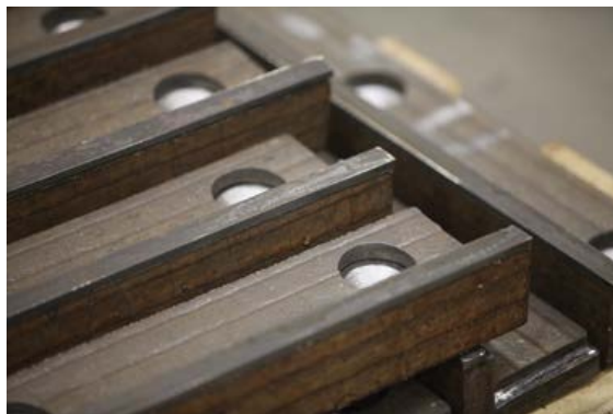
OEM parts fabricated by JADCO from Chromeweld plate.
