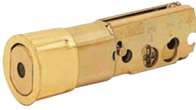
9093 Adjustable 2-3/8" or 2-3/4" backset drive-in for deadbolt latch
