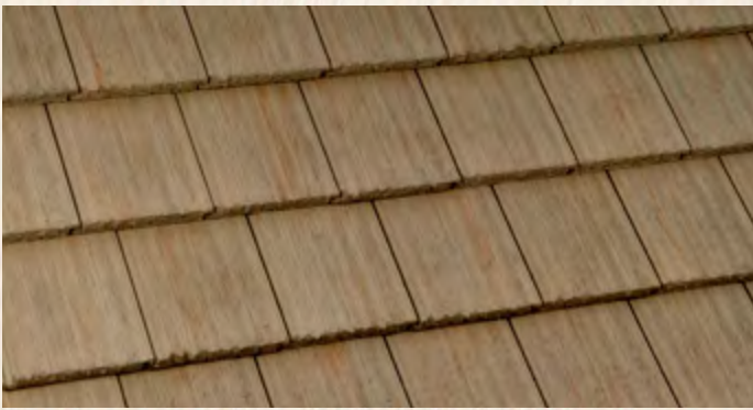
5530 Weathered Adobe - Hues of Tan, Rust Streaks T24 Ref: .23 Emi: .92 SRI: 24 A.SRI: 27 CRRC: 0918-0017
