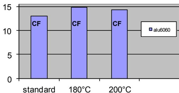
LSS: lap shear strength (MPa) with NF1465 .
