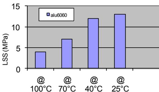
Lap Shear strength after weathering conditions
