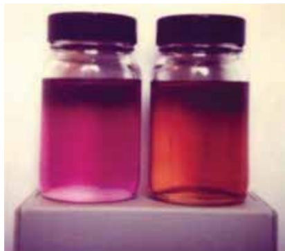
Figure 14.7 The first pure samples of C_{60} and C_{70} in benzene solution separated by chromatography at the University of Sussex. Reproduced from Ref. [3] with permission from The Royal Society of Chemistry. In benzene solution C_{60} is magenta and C_{70} on the right red.
