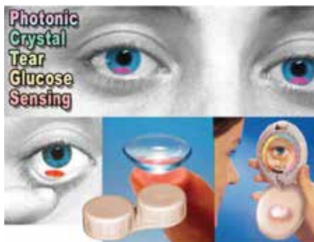
Figure 26.19 Conceptual drawing of photonic tear glucose sensing utilizing a mirror to examine the color of the photonic crystal sensor in the contact lens and compare the color to that of a calibrated reference color wheel. (Reproduced from Asher Research Group, Department of Chemistry, University of Pittsburgh, Colloid Group, http://www.pitt.edu/~asher/homepage/colgrp.html#pcca , accessed March 12, 2012. With permission.)
