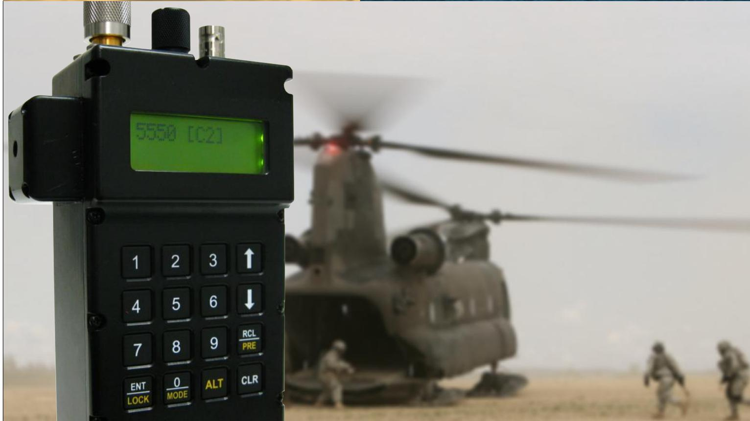
The MBT is a hand-held unit that transmits real-time, full-motion video. Designed to work over the L, S and C bands. It can be used to test all bands of the MVR-IV video receiver or any other video receiver. It can be operated stand-alone using the built-in keypad and LCD display or controlled via a computer.
