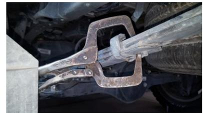
**Step 3:** After clamps have been placed remove the thick original 2<sup>nd</sup> stage leaf by removing the center bolt (new bolts comes with kit)
