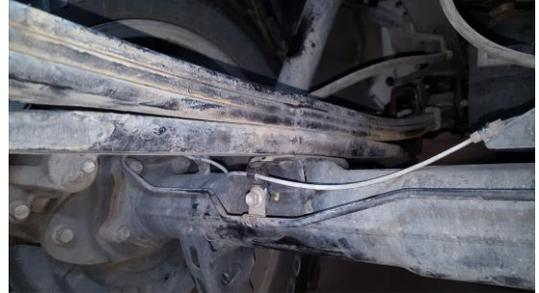
**Step 2:** Lift vehicle up in the rear off of the hitch receiver or off of the frame (cannot lift off of the axle) be careful to watch your brake lines and ABS lines while doing this. Img. 1
