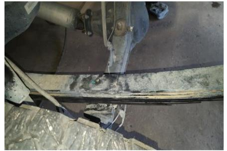
**Step 5:** Now that the 2<sup>nd</sup> stage is installed you can lower the vehicle back into the axle by lining the new center bolt up with the perch of the axle. After getting the springs in the axle you can put your top bump stop/top plate back on the spring and run the new U-bolts over the top of them.
