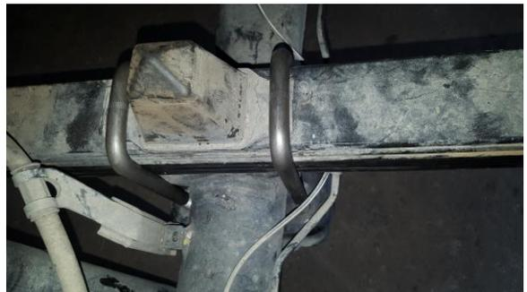
**Step 6:** Now that everything is in place you can put the bottom plate around the axle with the U-bolts sticking through, fasten the nuts on the U-bolts in a cross pattern torqueing them to 100- 124ft pounds. After U-bolts are tight you can re-lift your vehicle to make the shocks easier to hook up. Once shocks are tight installation is complete. (RE-Torque U-bolts after around 800 miles)
