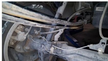
**Please note:** varying on the year some Tacoma trucks have an emergency brake line bracket to the stock second stage leaf, this needs to be removed, the new BSW build-up will have a new band clip to attach the existing bracket to.
