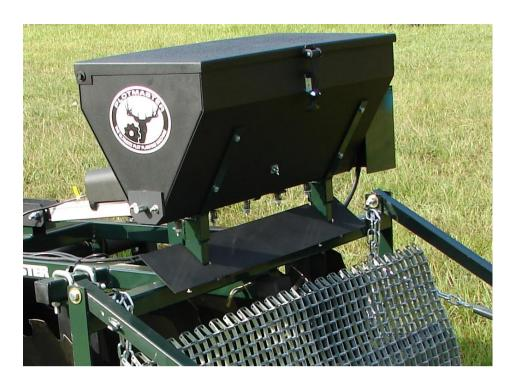
THE "SPLATTER PLATE" IS DESIGNED TO ALLOW SEED TO SCATTER AND SPREAD EVENLY.
