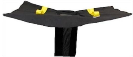
The material used in the Hornet's Nest drain inlet filter includes a nonwoven geotextile (skirt), as well as a woven geotextile (collection tube). The strapping is constructed from weather resistant 2" polypropylene webbing. The Hornet's Nest drain inlet filter is available in: 36" x 48" - 60" x 60" (custom sizing available).
