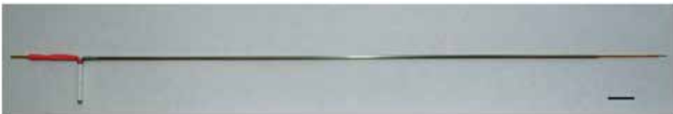
Figure 45.3 Electrophysiology targeting electrode. The exposed tungsten tip is at right (though too small to see at this resolution), the electrical contacts at left. The red contact at left is connected to the tungsten tip, while the white contact at left-bottom is connected to a stainless-steel jacket coaxial with the tungsten tip. In use, this electrode is inserted into the brain through a stainless-steel cannula, which is held in place by a stereotactic surgical frame. The black scale bar at the lower-right is 1 cm.
