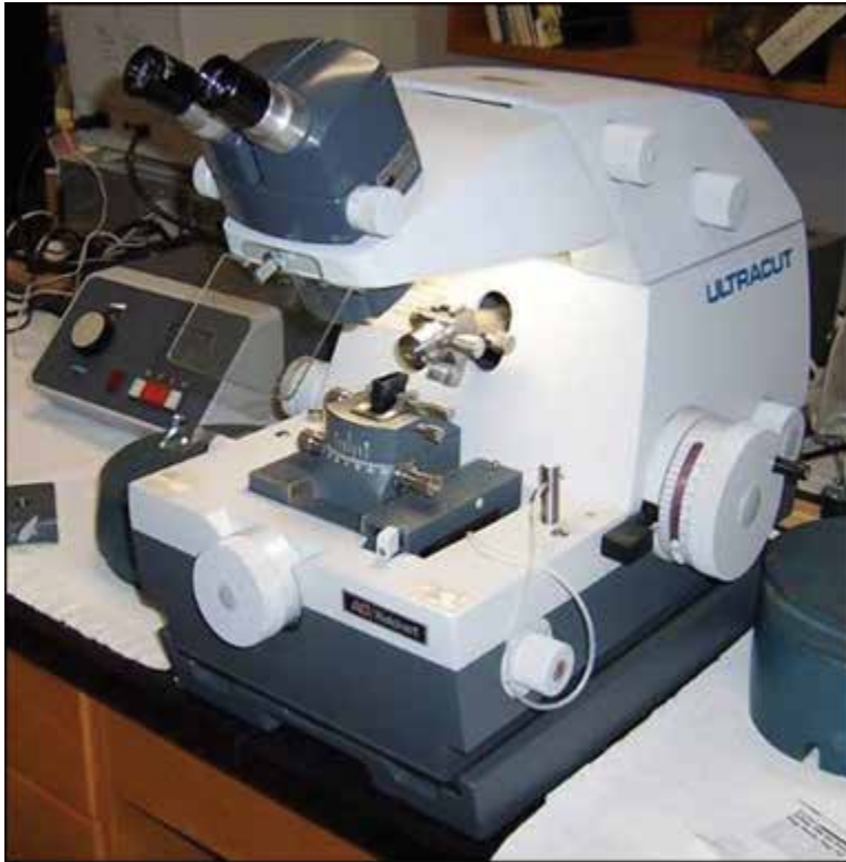
Sjöstrand's ultramicrotome. It dramatically improved ultrathin sectioning with minimal distortion. Courtesy of Prof. Dr. S. R. Bawa.
