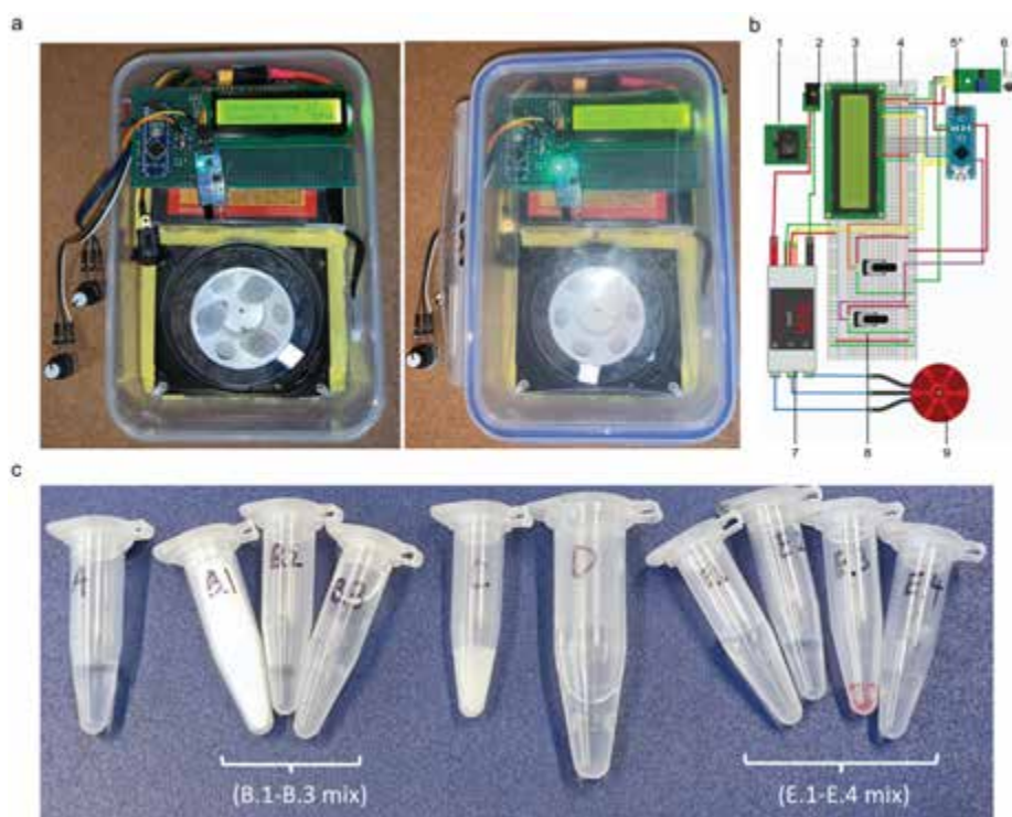
Figure 48.1 CentriDrive and reagents for LAMP assay. (a) The CentriDrive. (b) Circuit diagram of the CentriDrive. 1. Switch. 2. Power input. 3. LCD. 4. Breadboard. 5. Geekcreit Nano. 6. Infrared sensor. 7. ESC. 8. Potentiometer. 9. Motor. (c) List of all reagents for LAMP assay. Chemical A, Lysis/Inactivation buffer. Chemical B.1, NaI powder. Chemical B.2, 1 N HCl. Chemical B.3, Triton X-100. Chemical C, Silica binding suspension. Chemical D, 80% ethanol solution. Chemical E.1, PBS buffer. Chemical E.2, Primer solution. Chemical E.3, WarmStart® Colorimetric LAMP 2X Master Mix. Chemical E.4, SARS-CoV-2 solution. *The Arduino nano is shown in the figure due to limitations of the drawing software, but the Geekcreit Nano was used in the final test.
