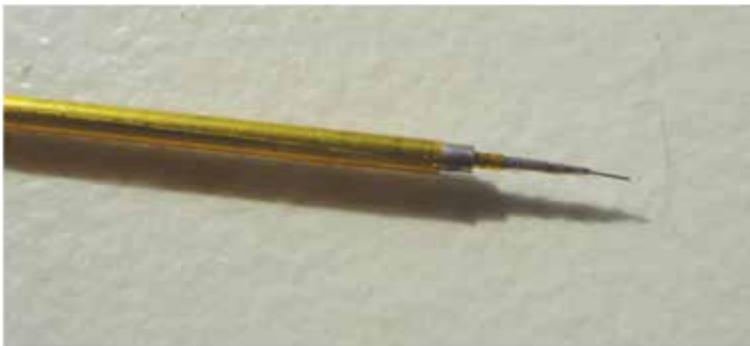
Figure 45.5 Carbon fiber electrode constructed by the Mayo Clinic Neural Engineering Laboratory. The exposed carbon fiber tip is at right.
