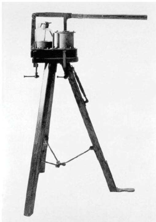
Lister's carbolic spray, nicknamed "the donkey," is shown above. It produced an aerosol of carbolic in the room, much to the discomfort of the surgeon and his assistants. This apparatus is preserved in the Hunterian Museum at the Royal College of Surgeons of England.
