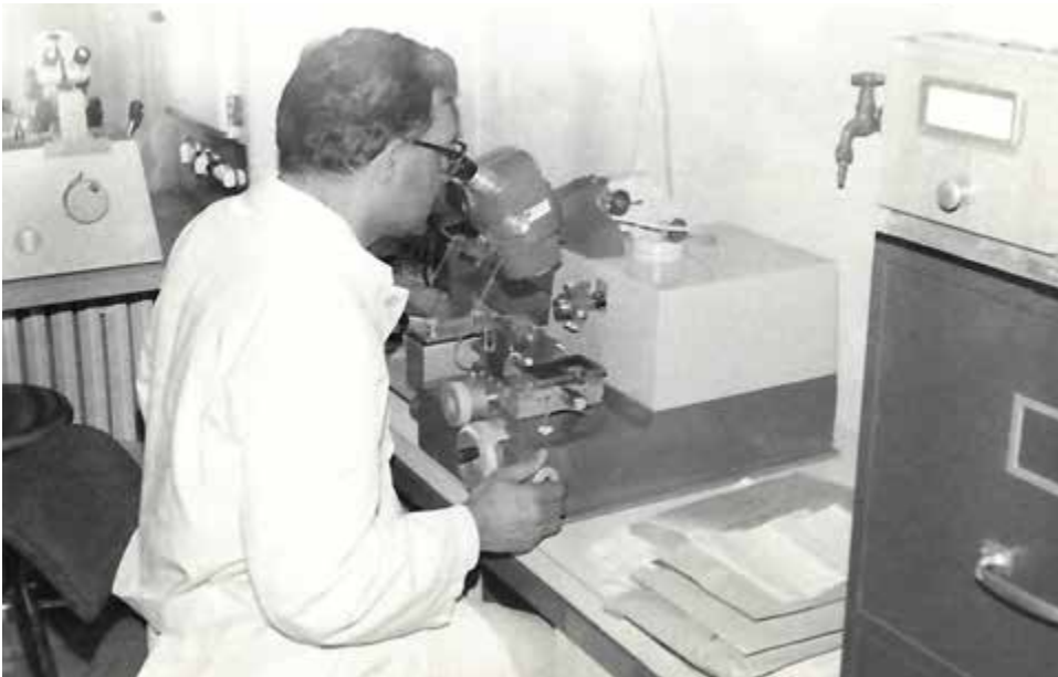
Photo 41. In the Electron Microscope Laboratory on an ultramicrotome, sectioning embedded biological tissue in preparation for microscopic examination.
