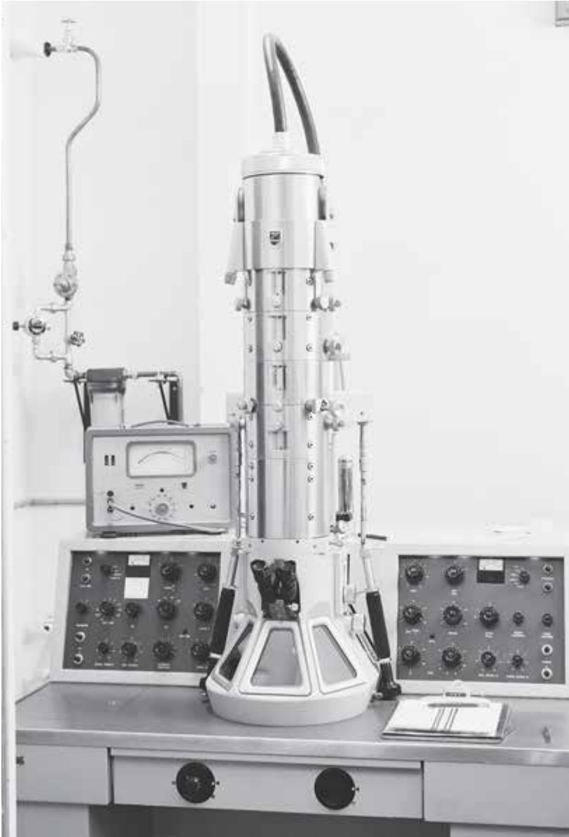
Image 7. This historic 1965 image depicts a transmission electron microscope (TEM). This remarkable instrument uses a beam of electrons that passes through an extremely thin specimen and on to an imaging surface. Rather than having a glass lens focusing the light (as in the case of a light microscope), the TEM employs an electromagnetic lens which focuses the electrons into a very fine beam. Sometimes a fluorescent surface is used, and at other times a sheet of photographic film, or in the case of modern-day technology, a digital camera captures the image. The electron microscope can reveal details that are tens of thousands of times smaller than can be seen by even the highest quality light microscope. TEMs can magnify objects up to 2 million times. Image courtesy of the Centers for Disease Control and Prevention.
