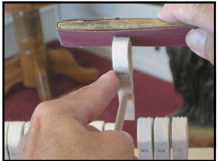
Hammers being filed to remove cut marks.
